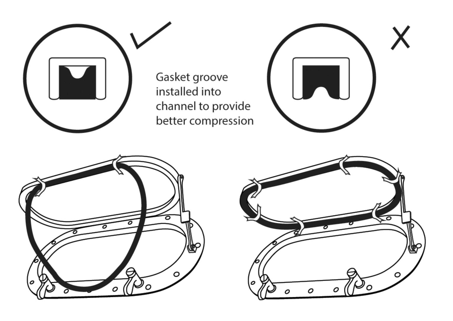
Clean portlight channel by scraping with a narrow scraper or screw driver, then wire brush to remove old gasket and adhesive. Use a marine grade urethane adhesive/sealant and apply a single bead into metal channel. Use tape to hold new gasket in place while adhesive cures. Close portlight and adjust hold down dogs for a tight seal. Inspect to make sure that gasket is centered in channel.
